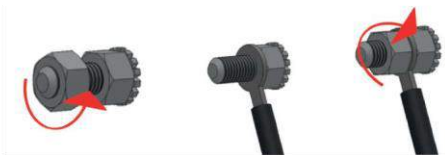
Connecting the unit to an electrical equalizing system
